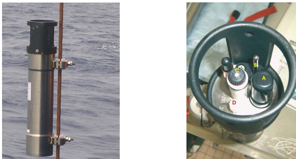
Fig. 1.4.2.1: MAPR mounted on a hydrograph wire (left) with sensors (right): nephelometer LBSS (A), temperature (B), Eh (C), and density (D), instrument from Dr. Edward Baker at NOAA Institution, Seattle USA. Eh-sensor from Dr. Nakamura, Tsukuba, Japan.
