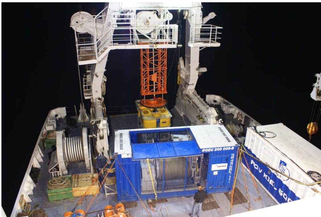
Fig. 1.4.10.4: Position of the ROV winch container, the control van, the ROV and its deployment frame at the rear of l'Atalante's working deck. The winch to the left hand side of the ROV winch was used to pay in/out of the lift line to lift the ROV (Foto: A. Massol, Ifremer).
