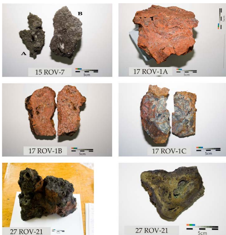
Fig. 1.4.5.1: Geological samples recovered during ROV stations: 15 ROV-7a: pyrite and markasite rich massive-sulphide with traces of anhydrite; 15 ROV-7b: massive anhydrite and pyrrhotite; 17 ROV-1a,b,c: strongly altered serpentinites, hematite impregnated; 27 ROV-21: chimney piece, collected at QUEST site, composed of chalcopyrite with Fe±Zn-sulfide rich outer layers.
