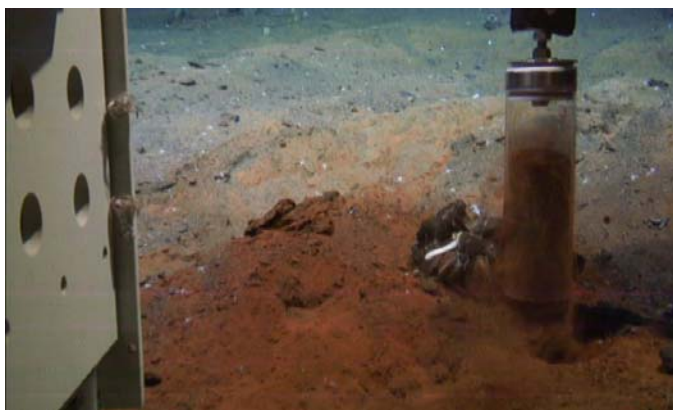
Fig 1.4.9.1: Sampling of sediment cores with a push corer and temperature measurement at the site Quest.
