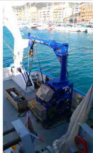
MVP200 installation on the Téthys II deck.
