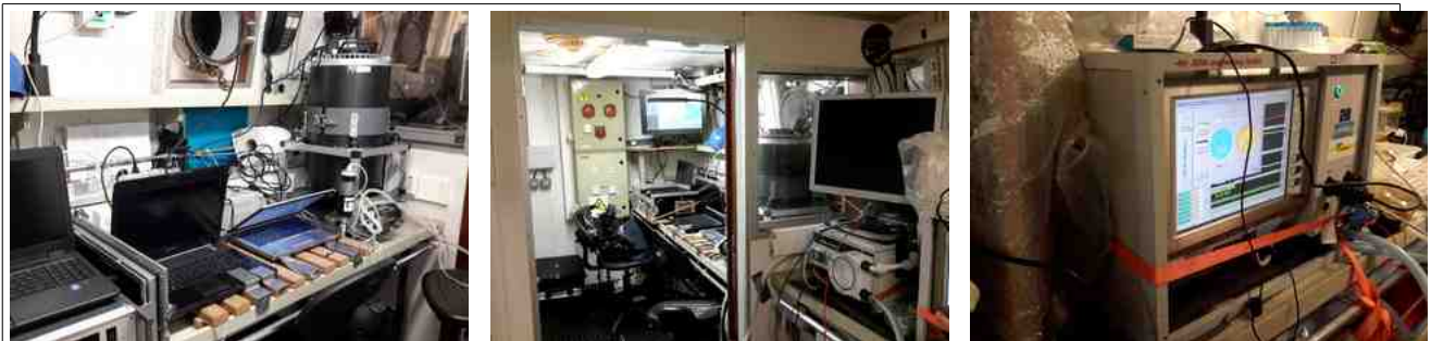
Picture of the Téthys II wet lab during the cruise with the sensors for the TSG+ sampling: Automated flow cytometer (left); pCO 2 (center); Pocket Ferry Box (right).
