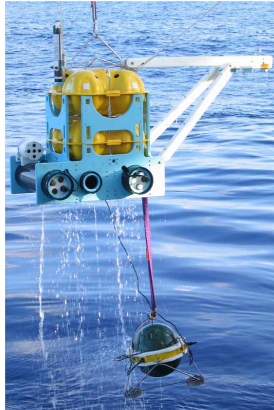
Fig. 4.2 Photographs of an INSU-IPGP OBS (above) and broadband OBS (right).
