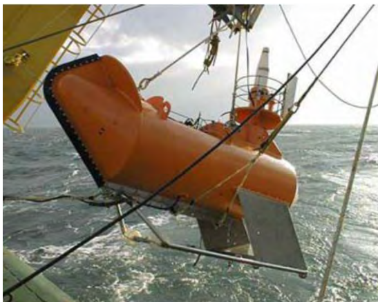
Figure 23 - Tail buoy towed at the end of the streamer
