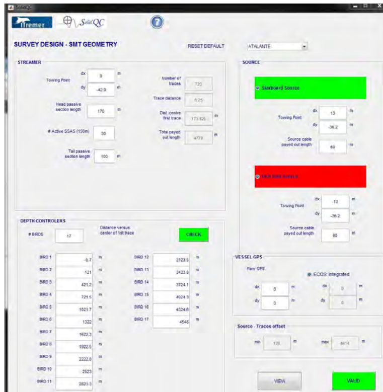
Figure 28 - The main input window for survey design information in QC-Solid. Streamer geometry is entered in the top left panel. The bottom left panel shows the distance along the streamer of the birds. The top right panel shows the x and y offsets from the centre of the array to each of the gun arrays, starboard and port sides. The boat GPS and navigation system offset, and the first and last trace offsets are shown in the bottom two right panels respectively.
