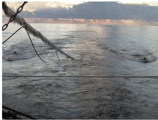
Figure 21 - Streamer towed behind the R/V L'Atalante. Also visible, attached to the main electric cable of the streamer, is the auxiliary cable used for the Passive Acoustic Monitoring System (PAM), employed for the detection of marine mammals.
