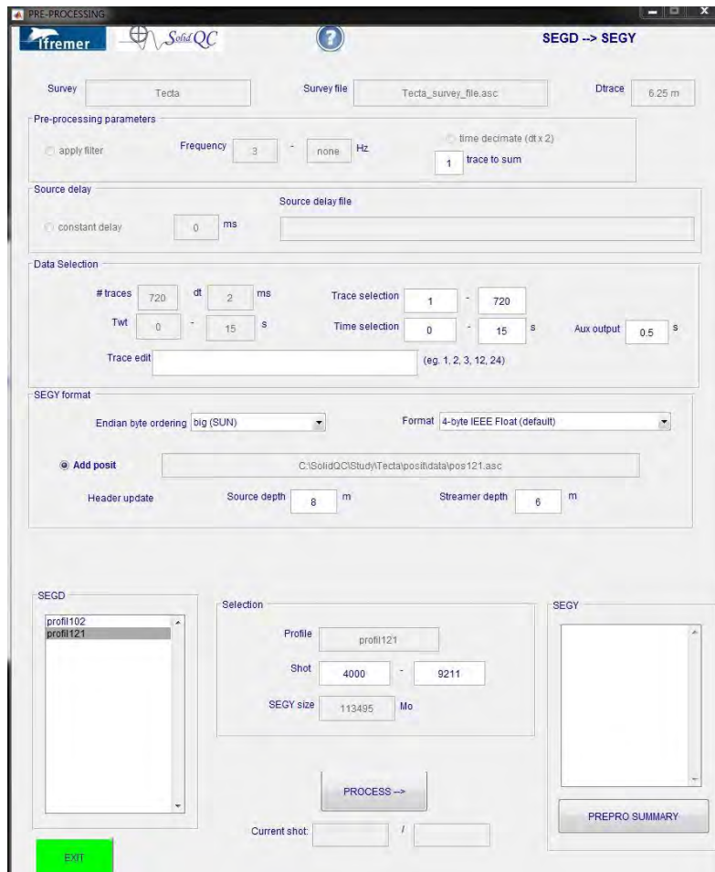
Figure 32 - Writing SEG1 shot gather files with geometry in the headers. At this step the position file containing shot, receiver and CDP, numbers and bin positions is written. The input files are the profile SEG1 data and the position geometry file posXXX.asc which was generated by combining survey and observer geometry information using QC-solid (see section 2.1.2).
