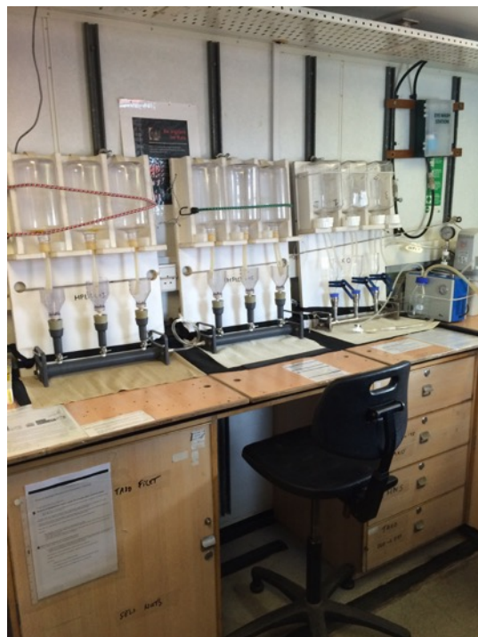
Fig. 3.4.1. Filtration system for a) pigment (HPLC, LOV-UPMC) and taxonomy b) for CHNS used in the Chemical laboratory during the Wapiti cruise.
