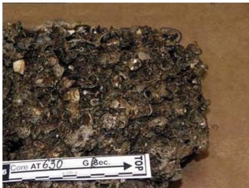
Figure 48. Carbonate-cemented chemosynthetic bivalves, which form extensive slabs on the seafloor, from TV grab AT630GR.
